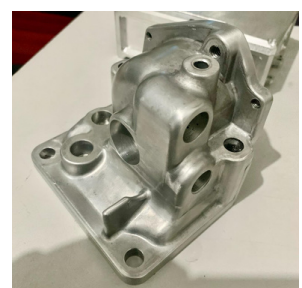
WATER OUTLET DIESEL
